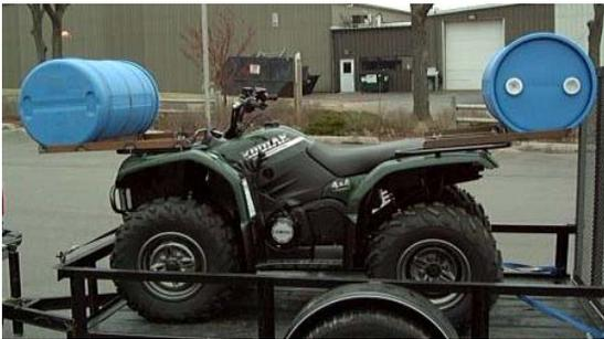
For patrolling the ice, two ATV's equipped with flotation devices are used. When the ice is unstable and unsafe, the staff uses the airboat, which allows them to move across ice or open water.
